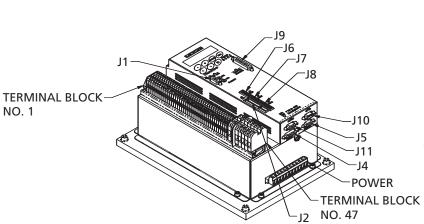
J1 **RS232 Communication** J2 Servodrive Enable and monitoring J4 Motor Encoder feedback J5 Motor Resolver feedback **Digital Input** J6 J7 **Digital Output** J9 Sin/Cos Encoder feedback (optional) J10 CAN in (or SERCOS/FireWire) J11 CAN out (or SERCOS/FireWire) POWER AC or DC power supply and motor
