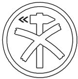
**Delicate part** (sticker on servomotor). A hammer must not be used to force the gearing or gearwheel onto the shaft when installing such parts. The screw thread in the center of the shaft must be used for this purpose. An extractor supported on the center of the shaft must be used when dismantling the parts. The permissible axial and radial forces **are in all cases exceeded** by the impulses due to hammering.
