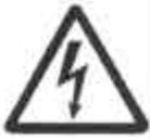
**WARNING** – You must disconnect the T200 Servo-drive from all voltage supplies (230 V.a.c., 120 V.a.c., 24 V.d.c.) before servicing.
