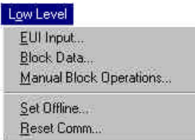
**EUI Input** - The EUI, or Engineering User Interface, provides access to individual servo-drive parameters, which, depending on user access level, may be read from or written to the drive.
