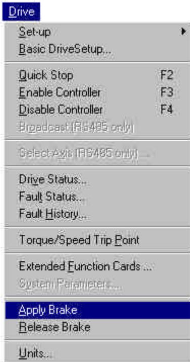
If an optional motor brake is fitted, this may be controlled from the **Drive Menu** with the **Apply Brake** and **Release Brake** commands.
