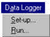
**Set-up** - All Data Logger parameters are entered in this dialog box. The user can define a specific trigger variable to the software which determines when the Data Logger begins the recording of data.
