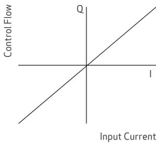
Minimal change in gain through null region. Best overall performance for most closed loop systems.
