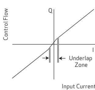
Null region flow gain is higher than normal. Always allows some small amount of flow past the spool.
