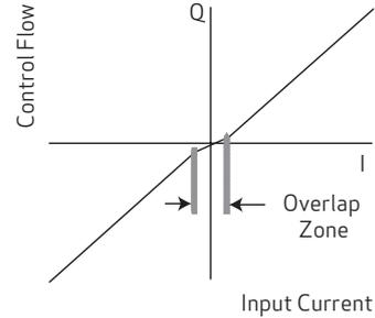
Null region flow gain is lower than normal. Spool types can range from minimal overlap to completely blocked flow.
