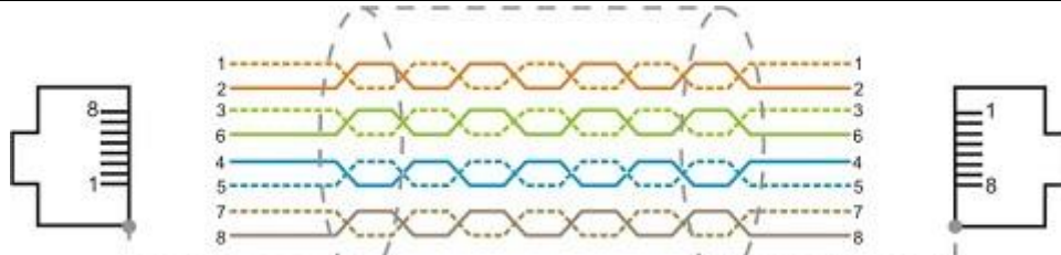
100BaseT Cable with Non-Crossed Twisted Pair Wires (Patch Cable)
