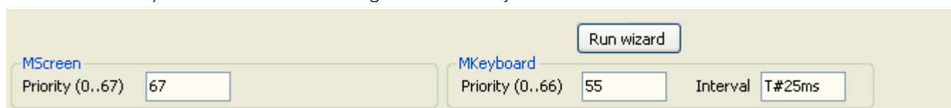
You can, before generating the video control, change the priority of the monitor thread, he priority of the keyboard thread and Interval. Expert users are required for this changes. The priority of the thread monitor is set from 0 (real time) to 67, while the thread of the keyboard is set from 0 (real time) to 66.
