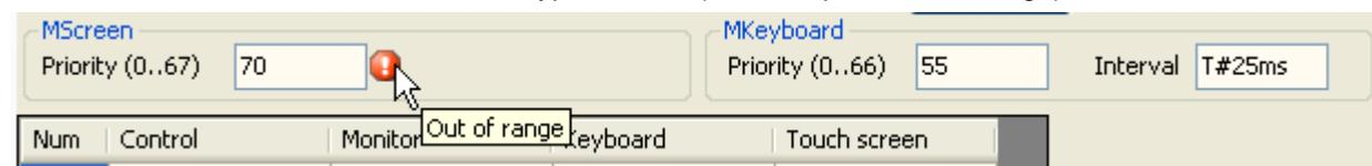
If you insert a wrong value in Interval field, will appear in the right side a white exclamation mark in a red field. Moving the mouse over the exclamation mark will be visible the type of error (for example: Invalid time base).
