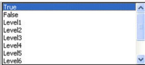
Level: can be set from Level 1 (High) to Level 10 (Low). The level is manage by the variable AccessLevel in the structure M\_Termln under M\_MC600Hmi library.
