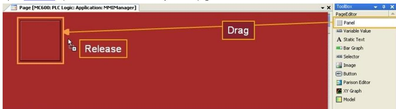
The inserted object will have the top/left coordinates respect to the mouse position. However is possible [move](#) the object created.
